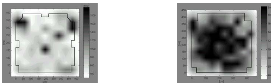
Fig. 38. Pulse Sonic Tomography of a S. Nicolò l'Arena pillar at different heights [Saisi, 2001].
